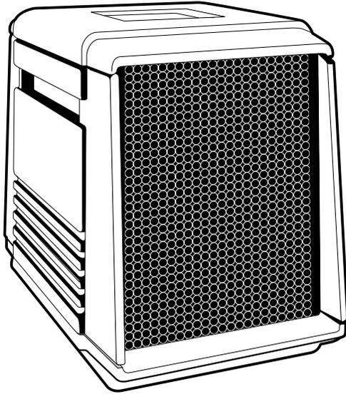
The Friedrich Electronic Air Cleaner is a self-contained console model consisting of a high voltage DC power supply, electronic cell, 3 speed fan, pre-filter and activated carbon post-filter in a rugged plastic cabinet.
